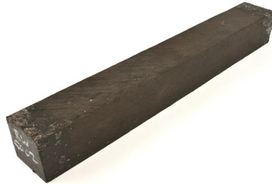
D. melanoxylon clarinet billet unfinished
