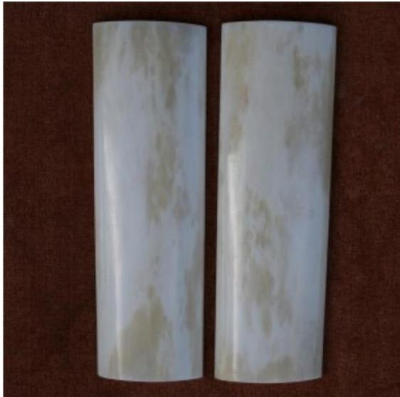
Bone scales cut from the metacarpals and metatarsals of a giraffe for the manufacturing of knife handles. Scales are approximately 159 x 49 x 12 mm in size.
