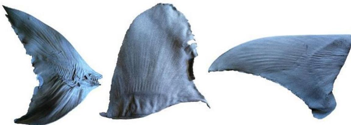
Figure 2. The replica shark fins after 3D printing using sintered nylon as the main material for printing (Bowmouth Guitarfish (*Rhina ancylostoma*) caudal fin, Oceanic Whitetip (*Carcharhinus longimanus*) dorsal fin, and Great Hammerhead (*Sphyrna mokarran*) pectoral fin)
