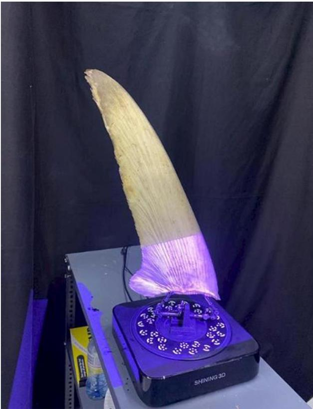
Figure 1. Blue Shark fin (pectoral) are 3D laser scanned using 3D image software. Photo: Markus Bürgener
