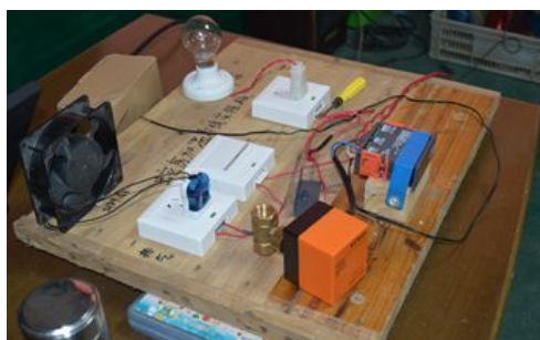
Fig. 10. A working electronics model provides a simple, low cost and effective means of teaching farmers how to control temperature in snake farms (Leicun Snake Farming School). This model could easily be explained in a 5 minute youtube clip.
