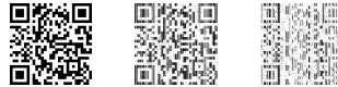
Figure 8 Minimum size normal QR code with 5 countries in three different deterioration levels (no deterioration, medium, and strong deterioration). For more examples, see Annex I .
