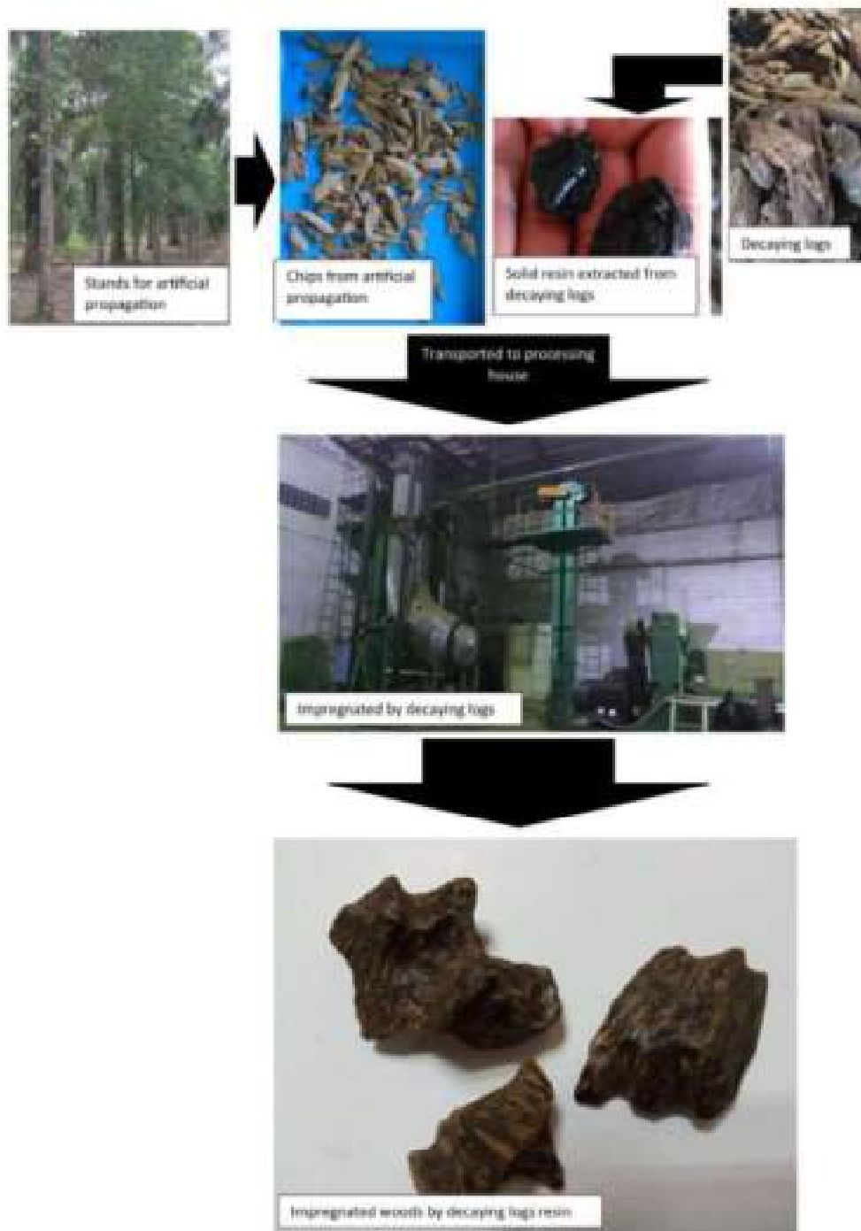
Figure 10. The processing of impregnated woods.
