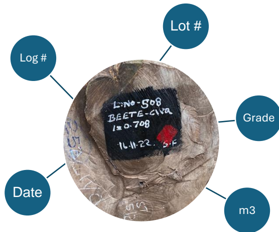
Figure 3.7 - Photo diagram of a log and the information stamped and printed on for traceability of forest compartment as well as for auction management.
