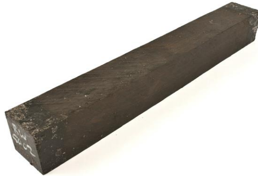
D. melanoxylon clarinet billet unfinished
