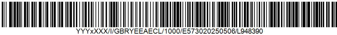
Figure 9 For comparison, a GS1-128 barcode encoding a CITES code with 47 characters. Note that normal mobile phones do not support reading this code.
