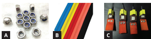
Figure 1. Materials for pangolin marking. Pan head screw A), Sling strap B) and radio transmitter C).
