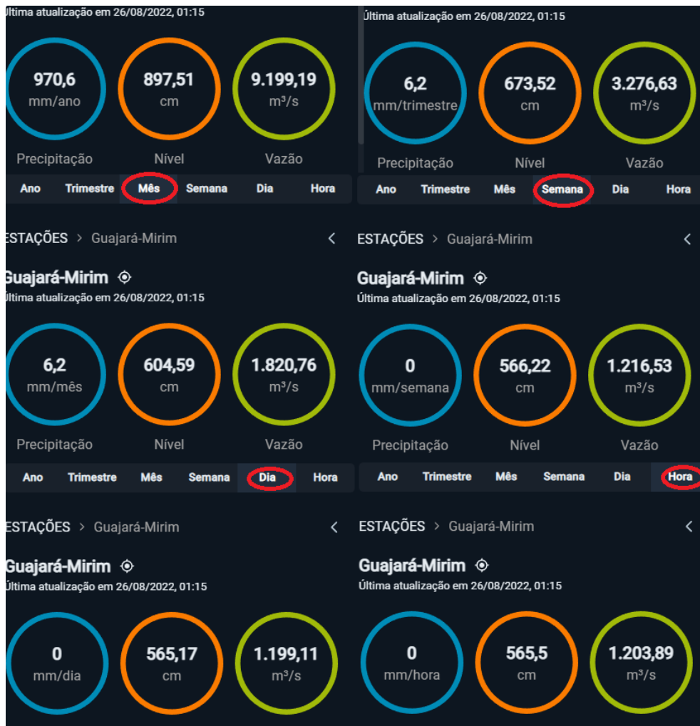
Figure 17. View of the geoviewer of the Amazon Networks Module showing in graphs the weekly real-time information from the Guajará-Mirim Station.
